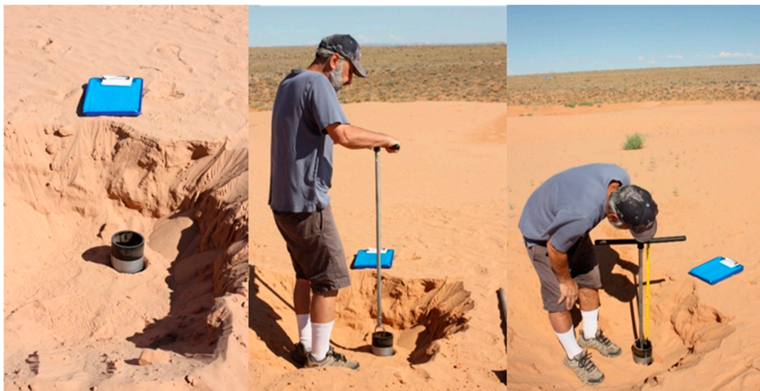
Figure 1. Hand-augering in Kanab Sand Dunes, southern Utah. Polyvinyl chloride (PVC) casing is inserted in top of auger hole to provide a reference platform for depth control and prevents influx of surface sediment downhole. The drill stem is advanced through the casing to the desired depth.
