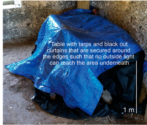
B) Subsampling core under in-the-field dark-lab
